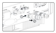
To disassemble the grid connectors from the SMILE5-INV, unscrew the grid connector counterclockwise until it can't be rotated and unplug it.
