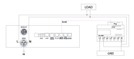
ADL-3000 single-phases Connect (without CT, with Meter plug)
