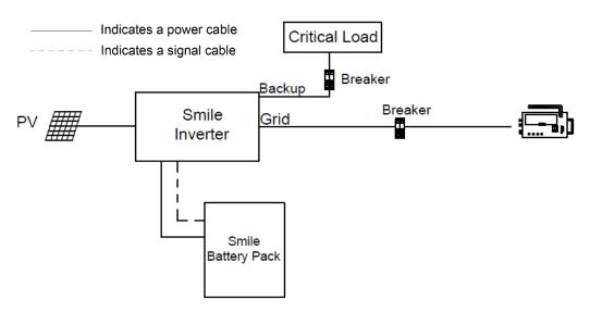
Off-grid (with Generator) Storage System-Scheme
