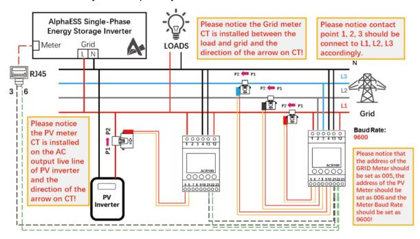
ACR10R three-phase Connection (AC- or Hybrid-Coupled System)
