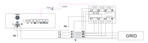
ADL-3000 three-phase Connect (with CT, without Meter plug)
