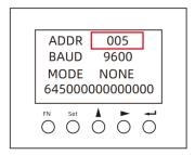
**Step 5:** Set the communication address and communication baud rate in the communication setting interface. When the meter is used as Grid meter (DC, AC/Hybrid system), the address is set to "005". When it is used as the PV meter (AC/Hybrid system), the address is set to "006". The baud rate is set to 9600.
