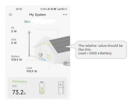
Step 2: Please switch on the PV switch on the energy storage inverter and the AC breaker on the PV inverter if there is any. Check the running status of the system.
