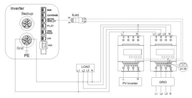
Wiring at three-phase feed in
