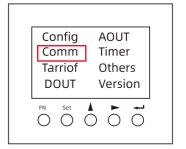
**Step 3:** Enter the password "0001" and confirm the entry by pressing the Enter key.
