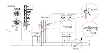
Wiring at three-phase feed in
